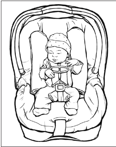
Figure 4. Car safety seat with a small cloth between the crotch strap and infant; retainer clip positioned at the center of the chest, level to the infant's armpits; and blanket rolls on both sides of the infant.
